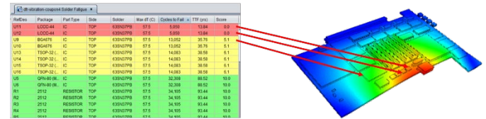
Figure 6: Reliability predictions can now be made at the component level, providing item managers and maintenance planners a deeper understanding of future repair requirements [17].
